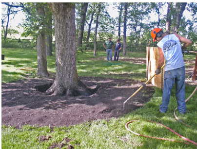
Depending on the treatment, organic matter may be added to the existing soil and incorporated in using the AIR-SPADE. This can greatly improve the quality of the soil for root growth.
