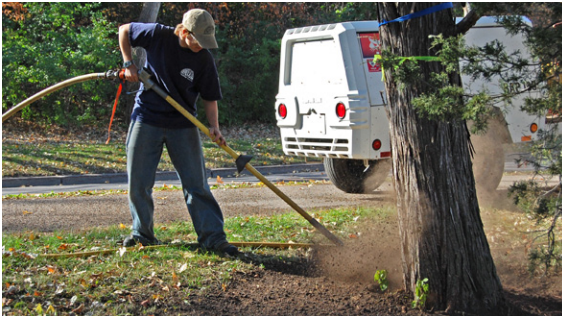
The AIR-SPADE is an air powered tool that allows an arborist to remove, excavate, or aerate soil without damage to sensitive roots.
